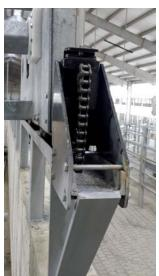
Track chain slips around the back of the stop and drops right onto the anchor's angled teeth for quick and easy removal chain slack. A few quick turns with a 3/4" wrench finishes adjusting chain tension.
